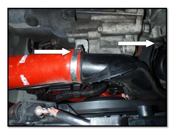
6. Remove the MAP sensor and install the boost take off block using the long screws supplied. Please note the cork gasket is between the pipe and the block, the boost take off is also closest to the plastic pipe as shown below.
