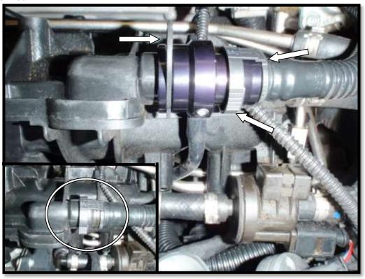
4. Using the bracket and one of the round spacers supplied install the solenoid/bracket as shown below. You will need to plug the supplied wiring harness into the OEM Diverter valve wiring harness, to do this you will need to reroute the wiring alongside the cam belt cover.
