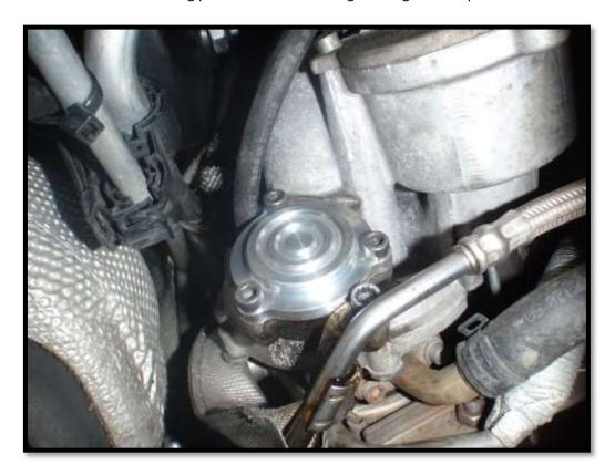
3. Unclip the breather and install the PCV take off, the take off should have two of the holes blocked off with grub screws unless you wish to fit a boost gauge etc. The other hole needs a vacuum take off with the largest hole screwed in. Secure the PCV take off with the small plastic clip supplied in the kit.
