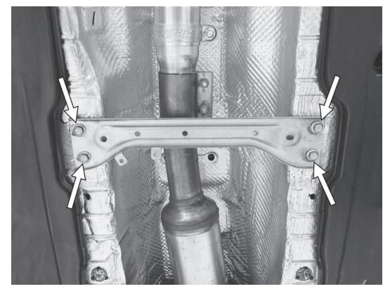
23) Install the front crossbrace onto the car. Tighten the four 13mm screws to 20Nm (177in-lbs).
